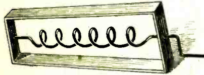
Fig. 3.—A Spiral Wire, the Shadow of Which, When the Wire is Rotated, Imitates a Series of Progressive Waves.
