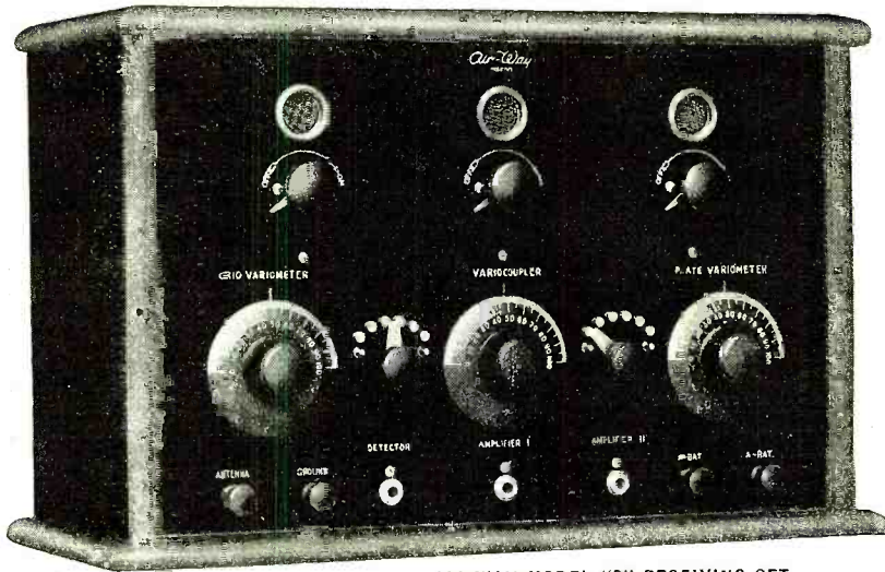
AIR-WAY MODEL "C" RECEIVING SET Here is a sound, practical set with detector and two stage amplification. It is remarkable for its long-range reception and its fineness of tuning.
