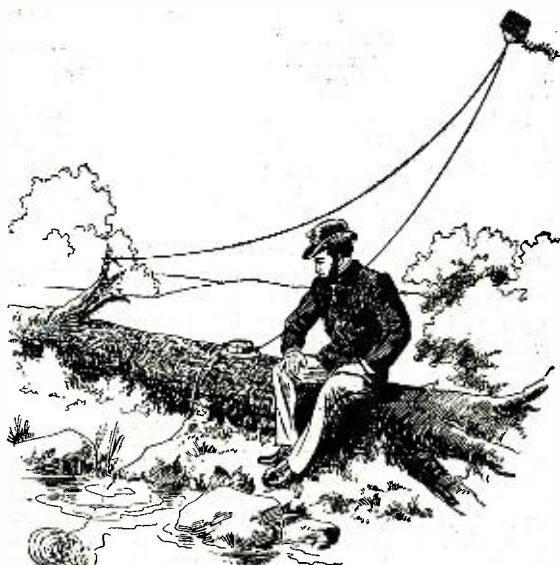
Copies of the Drawings Which Appeared in the Patent Papers of Mahlon Loomis. Left: Static Electricity Induced in an Elevated Wire Caused an Electrical Discharge. Right: At the Receiving End the Electrical Discharge Induced a Smaller Current in the Wire and Deflected a Galvanometer. Loomis Had Some Interesting and Visionary Theories of the Reasons for This Phenomenon.
