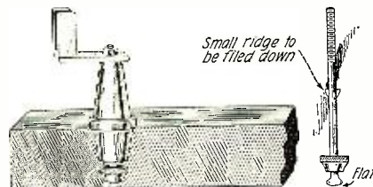
Discarded Spark Plugs May be Used to Improve the Standard Lightning Switch.
