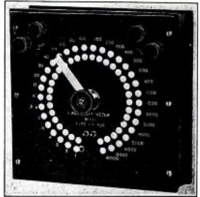
The Constant Impedance Audibility Meter. Note the Arrangement of the Switch Contacts.
