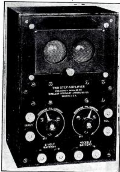
Fig. 1. A Commercial Type of Two Step Amplifier Designed by a Well-Known Expert Radio Engineer Which Helped Uncle Sam Win the War.
