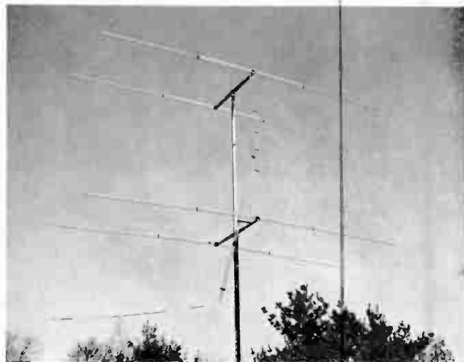
Fig. 5 Here is a simpler four-element array, the Vee-D-X type JR-13. Antenna has 72-ohm impedance and provides Q section
