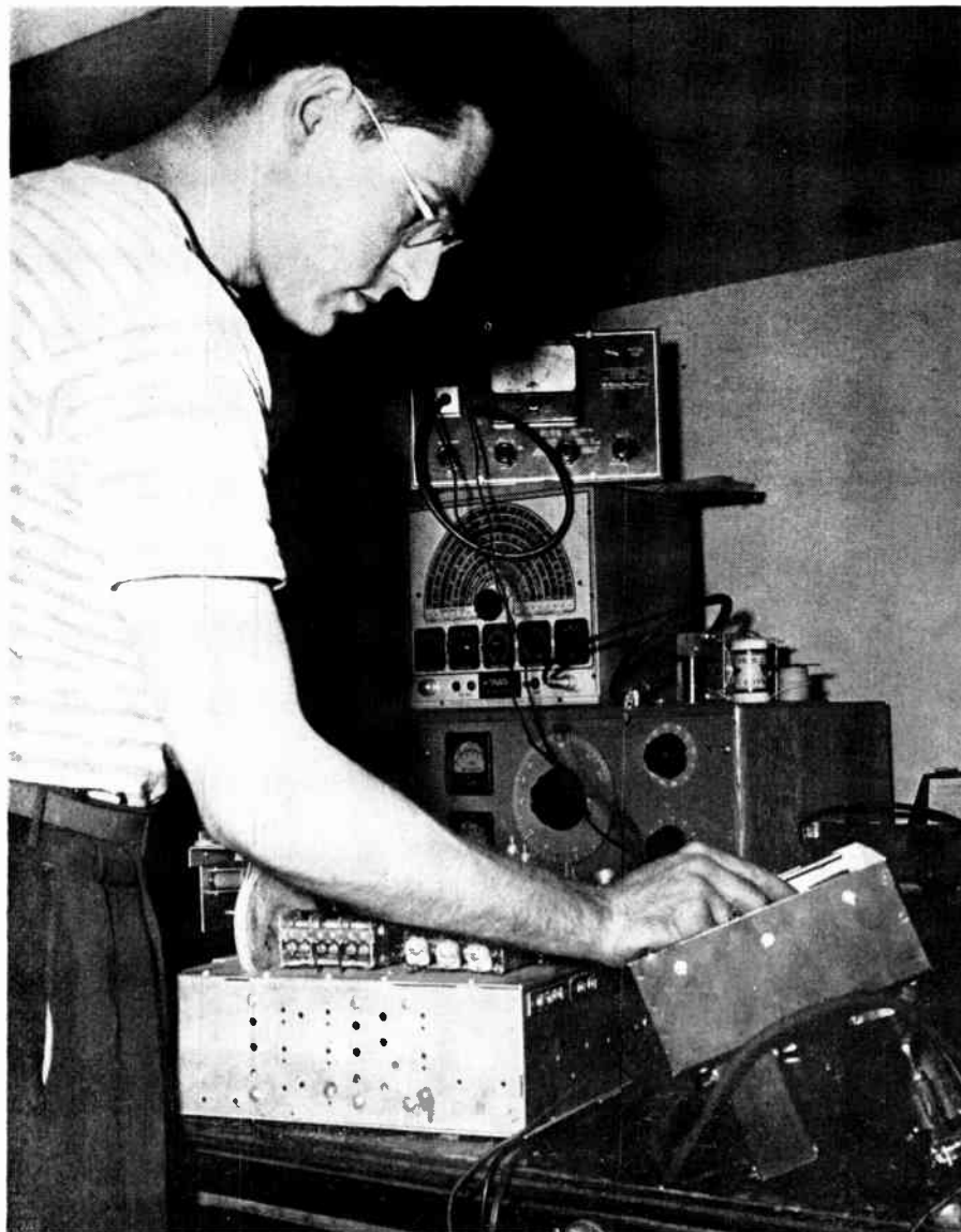
The completely assembled rig of amplifier, tuner, speaker and changer, plus pre-amp and matching transformer if necessary, should be thoroughly checked before mounting in cabinet. Here, a set of components is put on the test bench at Danby Radio Corp.
