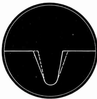
Fig. 6 Left: IF trace obtained by setting the oscilloscope to twice the power line frequency. Right: discriminator curves, 'scope at power frequency.
