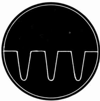
Fig. 5 Oscilloscope pattern obtained when the ratio of the oscilloscope sweep frequency to the sweep frequency of the generator is 2/3.
