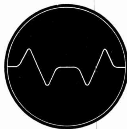
Fig. 6 Left: IF trace obtained by setting the oscilloscope to twice the power line frequency. Right: discriminator curves, 'scope at power frequency.
