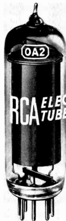
The OA2 miniature type regulates at 150 volts.
