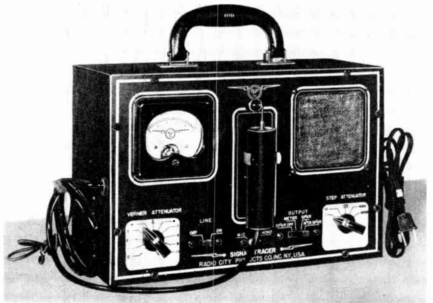
Fig. 8 A Radio City Products tracer which uses a detector probe.
