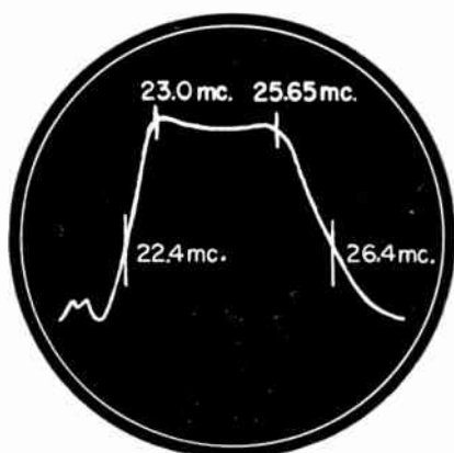
Fig. 5 Effect of sound traps on video IF response curve for G.E. Model 801 circuit.
