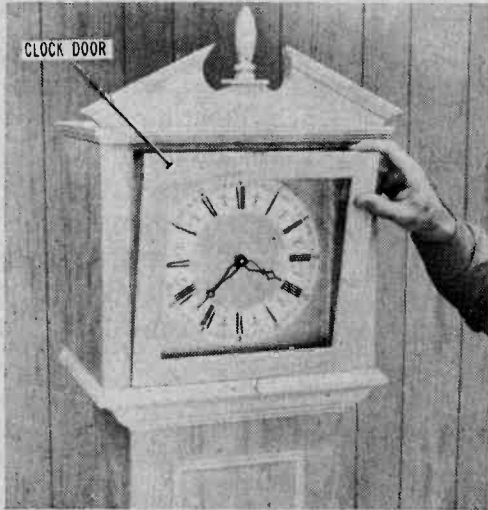
Dummy door (4) must be cut to fit opening, since it is glued permanently in place.
