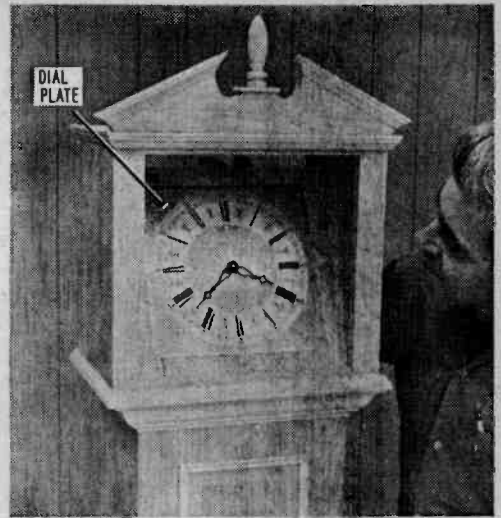
Dial and mechanism are mounted on 1/4-in. panel, then inserted through rear opening.
