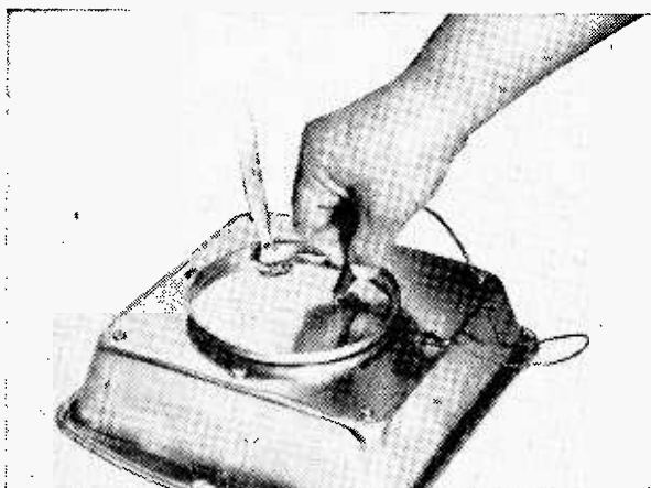
To charge metal disc, place it in center of plastic sheet, then touch center of disc with clip lead which runs to baking pan proper.
