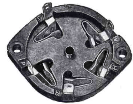
Bottom view without base showing contacts
