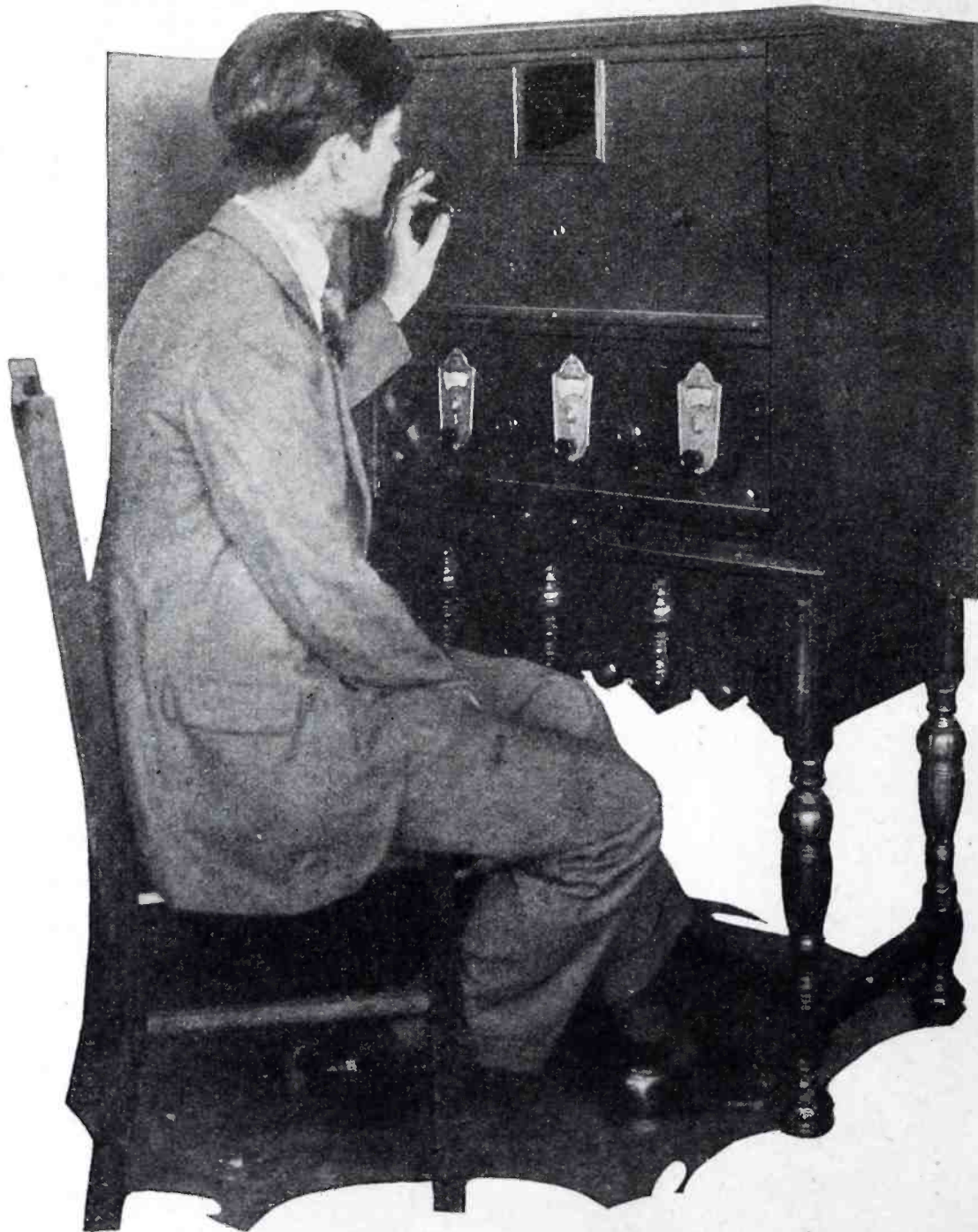
Operating the test receiver employed for demonstration of television reception from station WRNY. Directly beneath the scanning cabinet is an ordinary tuned R. F. broadcast receiver.
