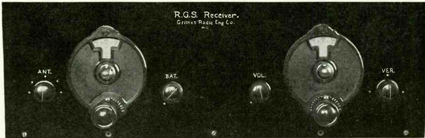
Front panel layout. The two large dials are the tuning controls while the knobs located on either side of both dials are clearly labeled for their use.
