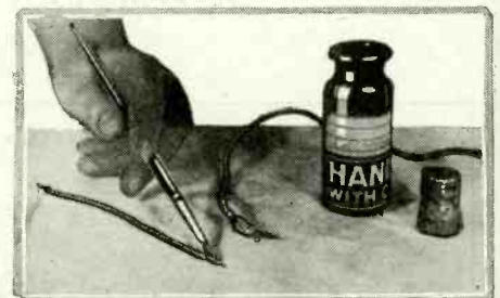
Collodion may be used to prevent fraying of cotton insulation.
