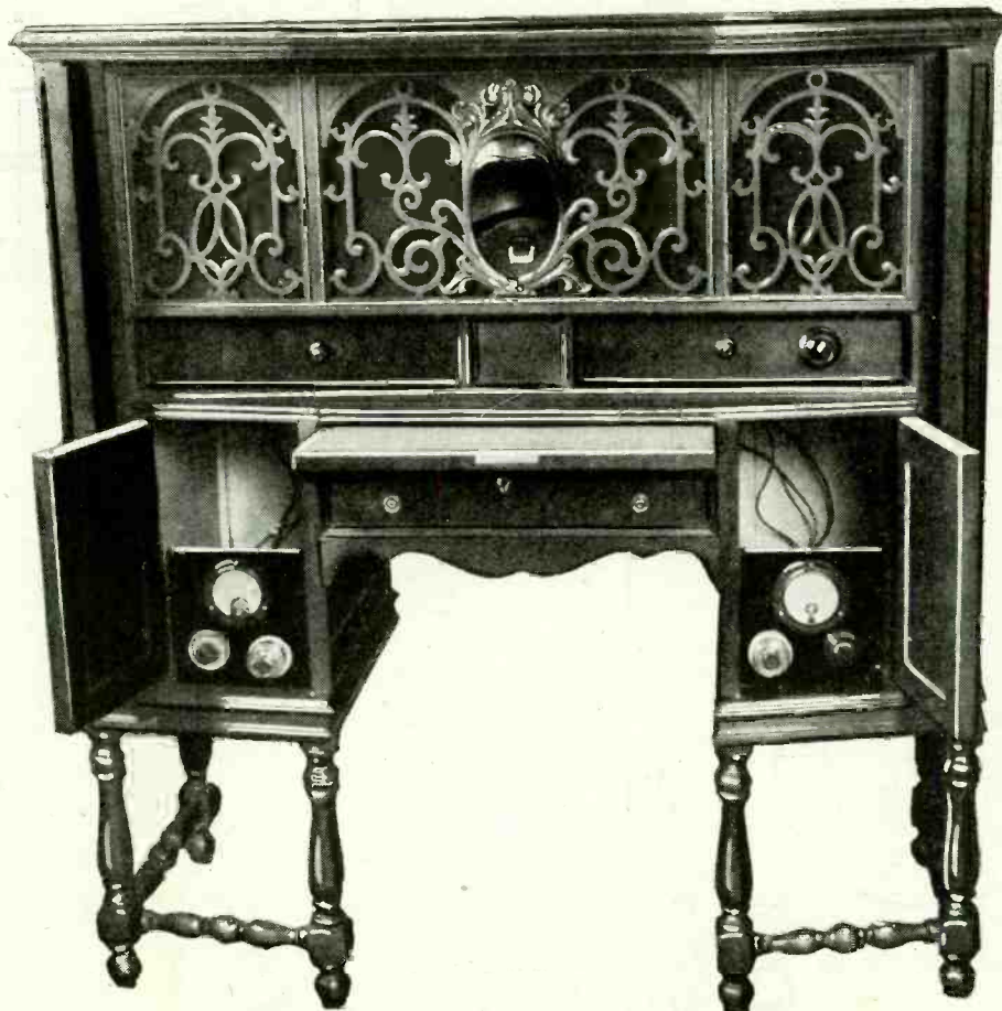
This shows the direct current eliminator installed in a De Luxe Super Zenith. The "A" section is at the right and the "B" eliminator is at the left.
