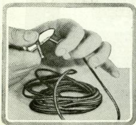
A sharp knife often cuts wire as well as insulation.
