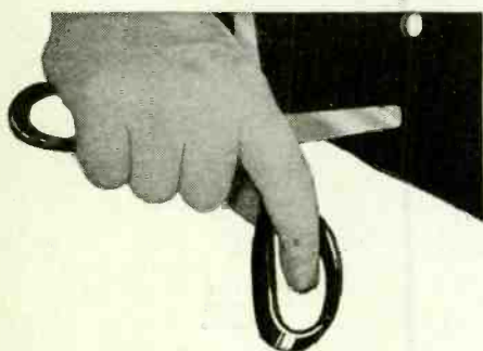
An ordinary pair of household shears used as a reamer.
