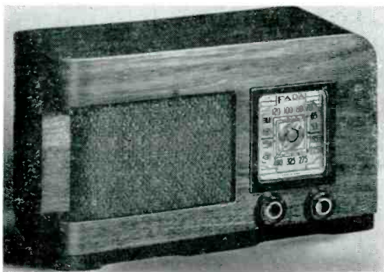
Above is Fada Radio's 6 tube superheterodyne 196 Model 1002. Set features walnut case, 8 tube performance, and a noise reducing RF stage. Automatic volume control and both AC and DC are also featured.
