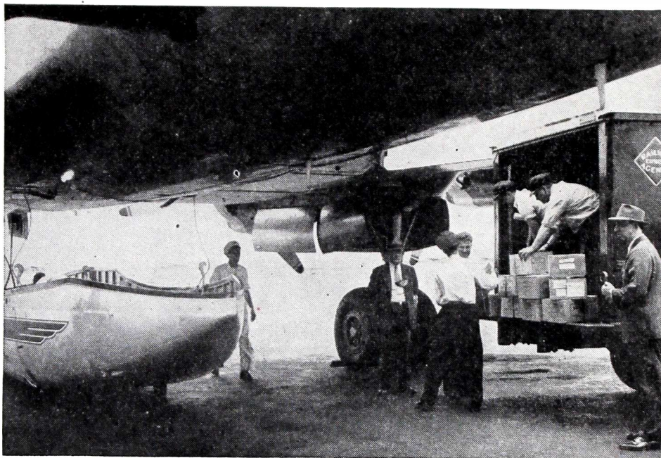
Pictured here is the scene at Newark Airport as 8,824 pounds of Emerson radios were air-expressed to Bared Bros. in Havana, Emerson Cuban distributor. Most of the 185 cartons were stowed in the newly-developed cargo "canoe", left, which is attached underside of Constellation fuselage when loaded. Shipment was handled by Air Division of Railway Express.
