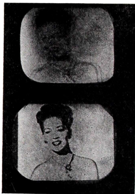
Picture on top shows reception of phone vision picture as seen on ordinary television receiver without the key frequencies. Picture below is from same transmitter but the key frequencies needed to unscramble the picture have reached the receiver by telephone wire.
