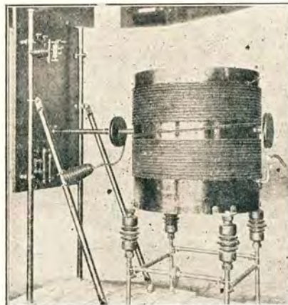
HERE'S THE VARIOMETER WE ARE GOING TO GET WHEN WE BUILD OUR FINAL SET. THIS IS A SIDE SLANT AT THE INTERMEDIATE CIRCUIT VARIOMETER OF ONE OF THOSE 20 KW BANANA ROUTE OUTFITS. IT MIGHT DO FOR A BATH TUB IF IT WERE FITTED WITH A BOTTOM.
