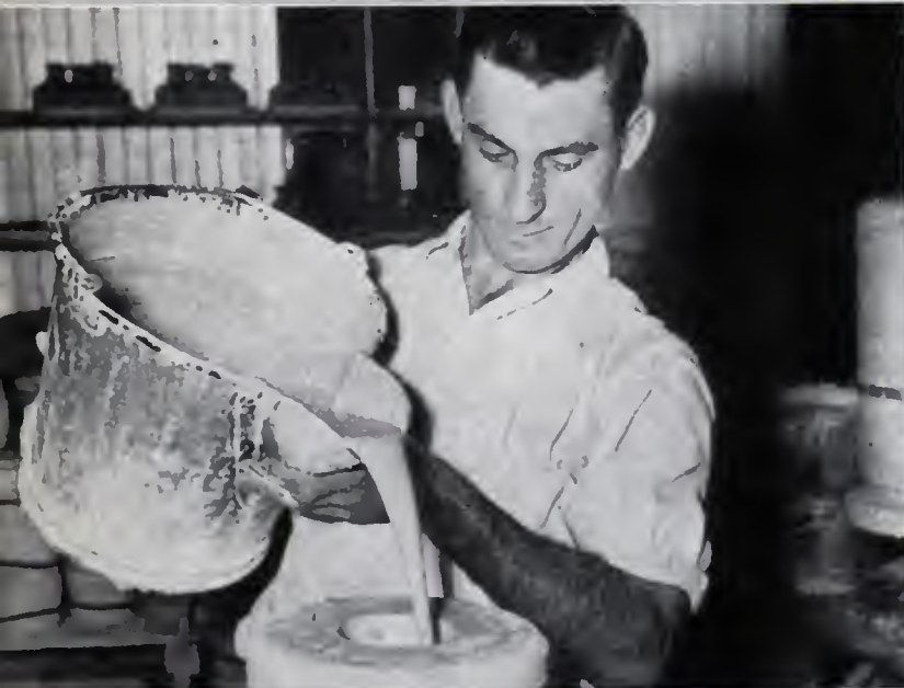
POURING YASE MOULDS In the hot, moist air of a Trenton, N. J., factory, this man is one of America's 167,000 pottery workers, thirty percent of whom are women. The potter's job, listeners learned, was old before Bible times
