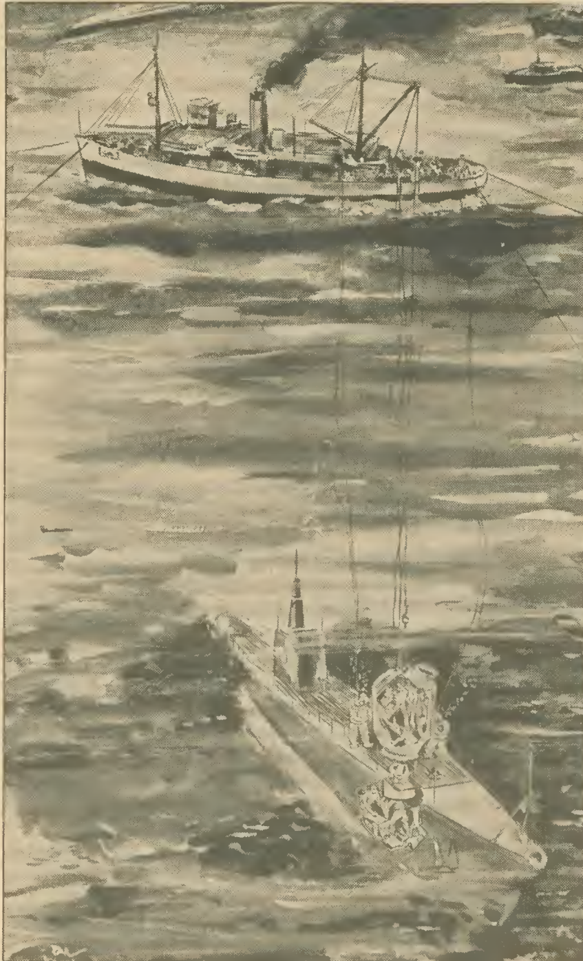
—International Above drawing shows how the miracle-bell was lowered from the Falcon on guide lines hooked by divers to the stricken Squalus 240 feet down. The steel bell fitted over an emergency hatch, enabling survivors to escape
