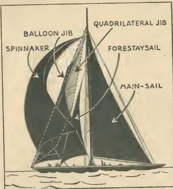
Sail Plan that will enable listeners to follow accurately the changes in rigging made by both contenders while the races are on (Courtesy of Ian McKinnis, marine architect)
