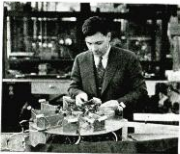
P. D. Zottu, of RCA Radiotron, with a model of the 120 cm oscillator employing eight tubes. This oscillator operates with an efficiency of 20 per cent.
