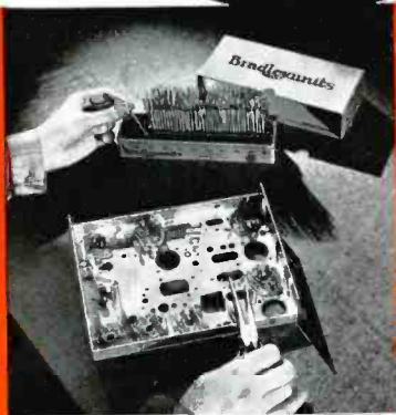
THE NEW WAY —Scientific packaging eliminates resistor fumbling and speeds up the production of radio equipment.
