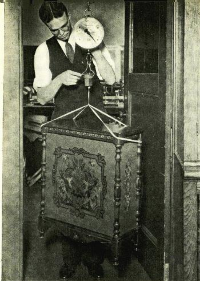
Alnico magnet sustaining pull of 60 times its own weight.
