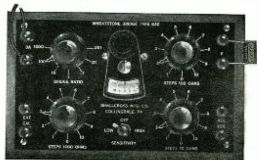
Fig. 1 Shallcross Wheatstone bridge.
