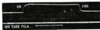
Fig. 3. 199 filament, .038 second. Can be protected by 1/4 amp. fuse, as can the T. G. above.
