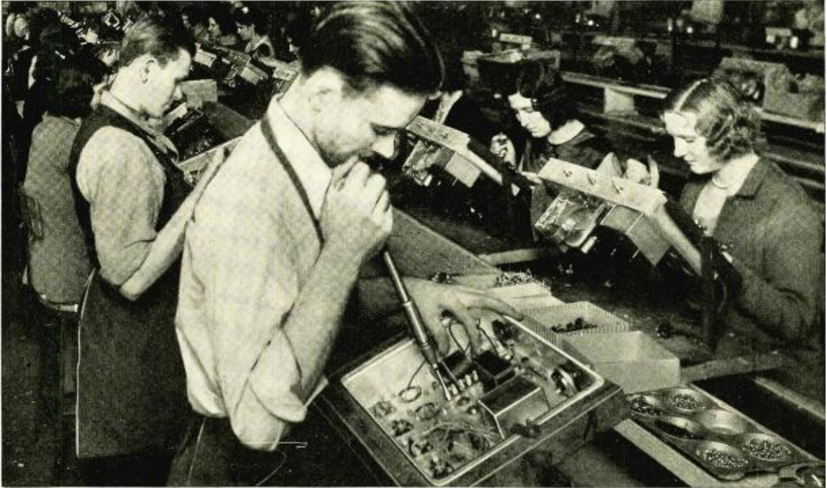
United Air Cleaner Corporation speedily run in Self-tapping Screws with spiral screw drivers.
