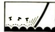
This is the action of the usual wire wound control after it has been in use for some time . . . like dragging a stick over a cobblestone pavement.
