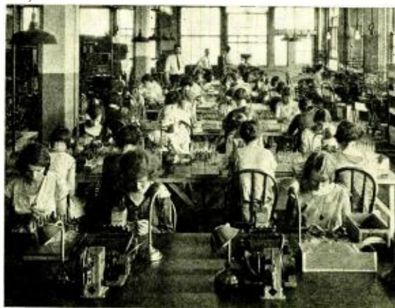
Fig. 1. Assembly benches where formed stem has plate, grid and filament attached.
