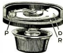
This shows the exclusive rocking disc construction of Centralab volume control. "R" is the resistance. Contact disc "D" has only a rocking action on the resistance. Pressure arm "P" together with shaft and bushing is fully insulated.
