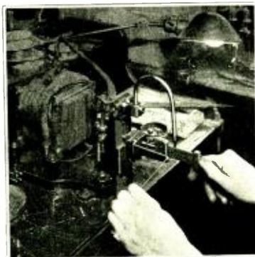
Welding molybdenum wire into vacuum tube grids in an experimental tube factory.
