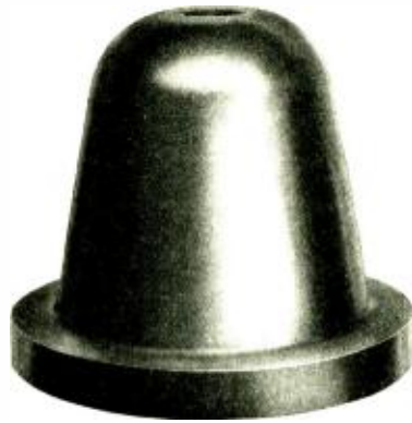
Textolite explosion chamber, 12 in. high, 14 1/2 in. diameter. Will withstand 1500-kv. and hydrostatic pressure of 925 lb. to sq. in.
