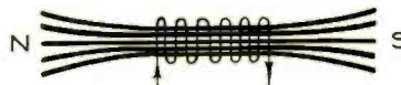
The laminations of an audio transformer are influenced by the current flowing in the primary winding and excessive vibration of the laminations in turn impresses a voltage in the winding corresponding to the movement.
