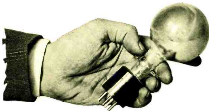
A General Electric PJ type, potassium hydride, central anode photoelectric cell.
