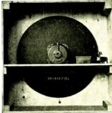
The scanning disc and driving motor used in the television receiver shown diagrammatically on the opposite page.
