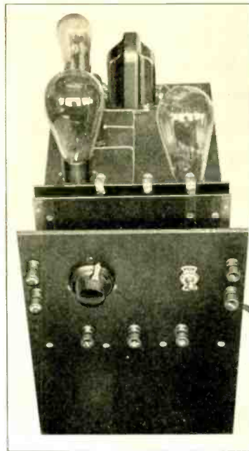
Front panel view of the Phonograph Amplifier. The knob controls the variable "C" bias resistor for the 227 tube.
