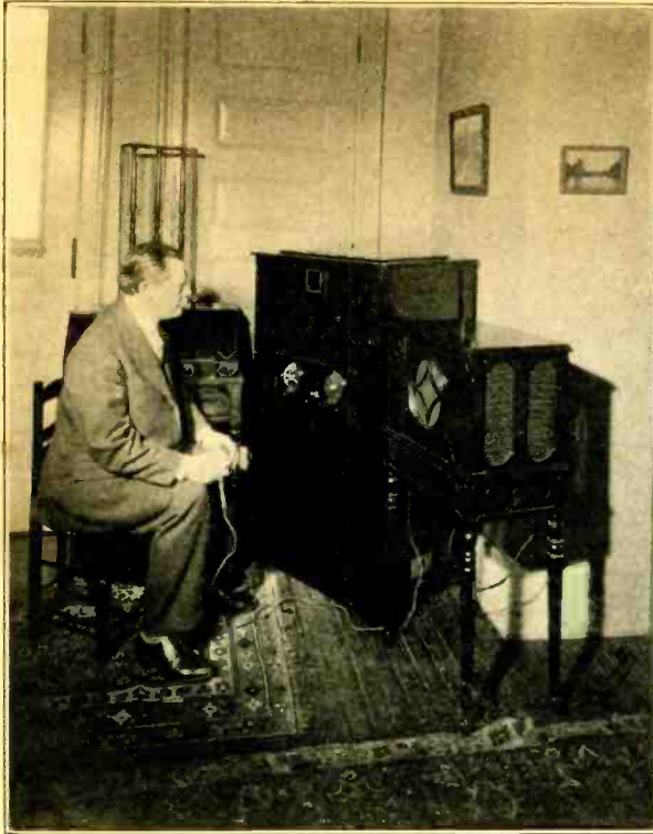
Dr. E. F. W. Alexander seated in front of his newly developed television receiver. The three-inch picture screen is seen near the top of the cabinet. Dr. Alexander is holding the push button which is used for maintaining the proper speed of the revolving "scanning disc."
