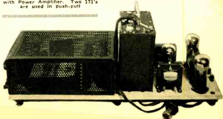
The completed Vitrohm D.C. Unit with Power Amplifier. Two 171's are used in push-pull
