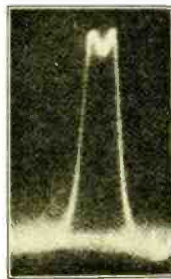
Fig. 4. Oscillogram showing the frequency characteristics of an actual band selector corresponding to Fig. 3. Carrier frequency, 635 kc. Effective band width, 18 kc
