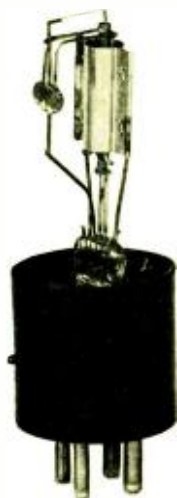
One of the A.C. tubes devoid of its glass enclosure. The heater element can be seen protruding from the top. The usual fifth prong common to A.C. tubes of this type, is eliminated by connecting the heater element to the negative leg of the filament. Receivers using these tubes can be operated from D.C. if desired without making circuit changes.
