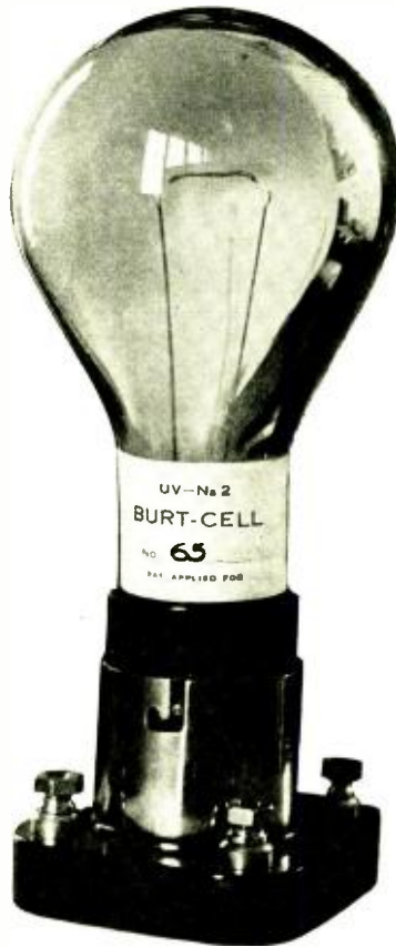
A high vacuum photo-electric cell without appreciable fatigue.
