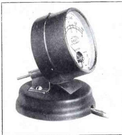
4. Used as a pin-jack voltmeter this Weston instrument reads up to 4 volts, on 160 volts when put into the mounting base which contains an extra resistance
