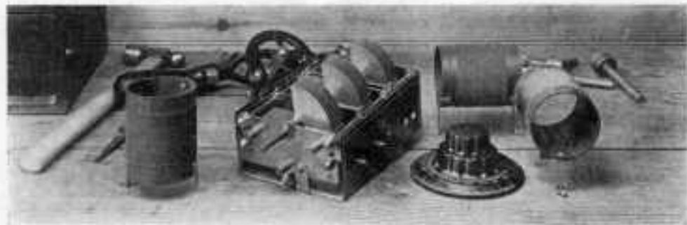
The Mohawk single-control construction kit consists of a triple condenser, vernier knob, and three R. F. transformers
