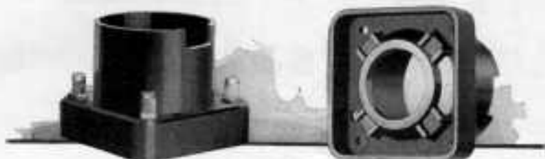
The completed Caldwell Socket is shown at the left. At the right is the one-piece Bakelite molding ready for insertion of contact springs. The spring construction differs from the usual practice in that these pass through slots in the central ring, making contact with the sides and not the bottom of the tube pins. Sockets manufactured by Knox Corporation, Galeburg, Ill.
