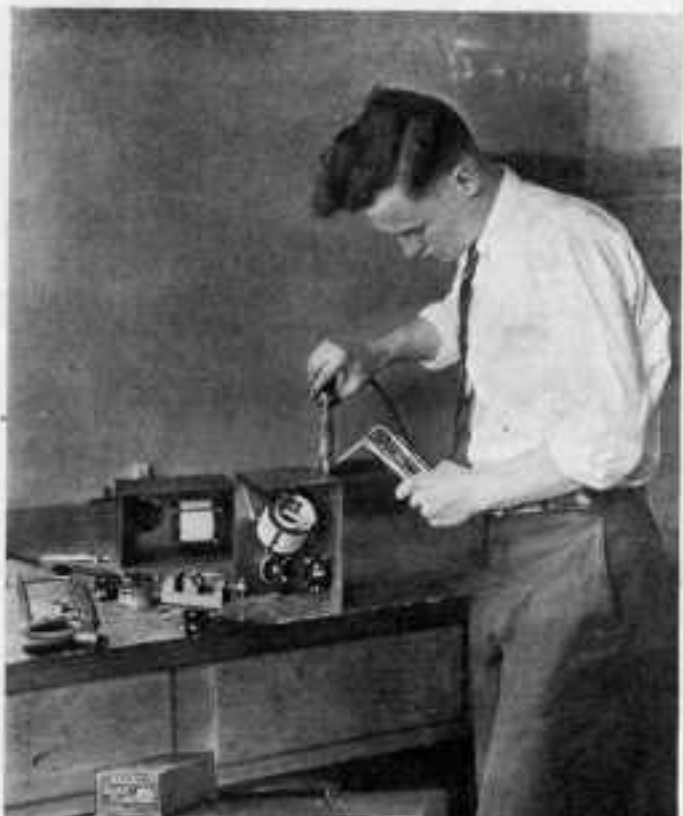
Figs. 3 and 4. Because the heat was conducted away so rapidly by the large area of the brass sheet, it was necessary to melt the solder with an electric iron while the brass was heated with an alcohol torch. The parts were mounted on the front and back before the shield was soldered together.
