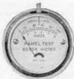
Throwing the little switch makes the Beede meter show the filament or plate voltage.
