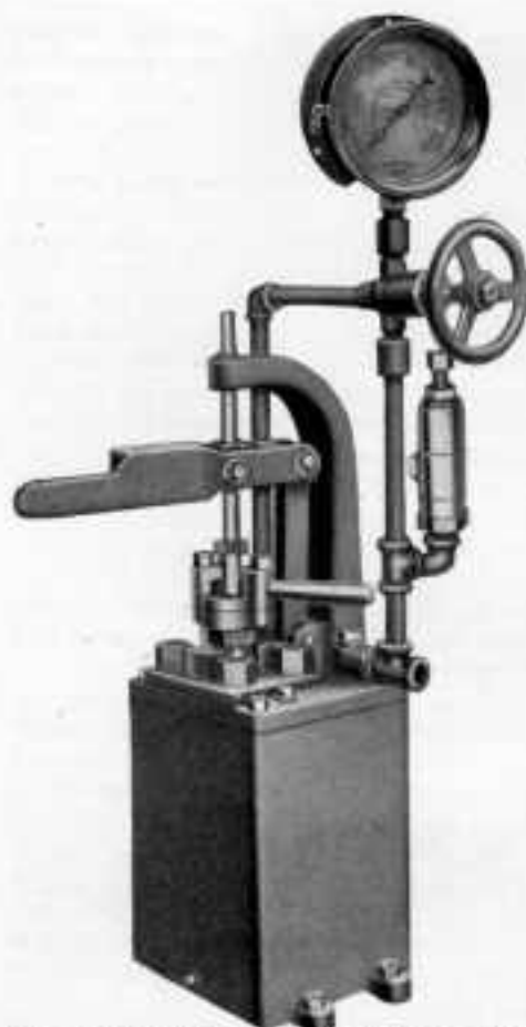
Fig. 3. Half a dozen strokes with the hand pump and full pressure is applied to the press. A reservoir is provided, so that the same water is used over and over again.
