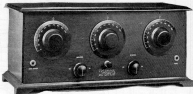
Inside and outside views of the Freshman five-tube tuned R. F. set which employs a non-oscillating circuit system.
