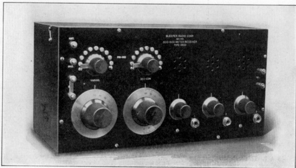
Fig. 1. Compact, sturdy, and reliable is this loosely coupled receiving set, shown here ready to connect for operating
