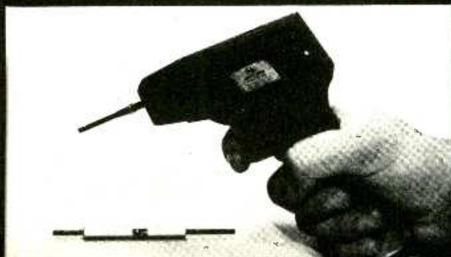
THE WIRE-WRAP GUN spins the wires on fast, but that’s all it does, at considerably greater cost than the small hand tool that wraps, unwraps, and strips the insulation.
