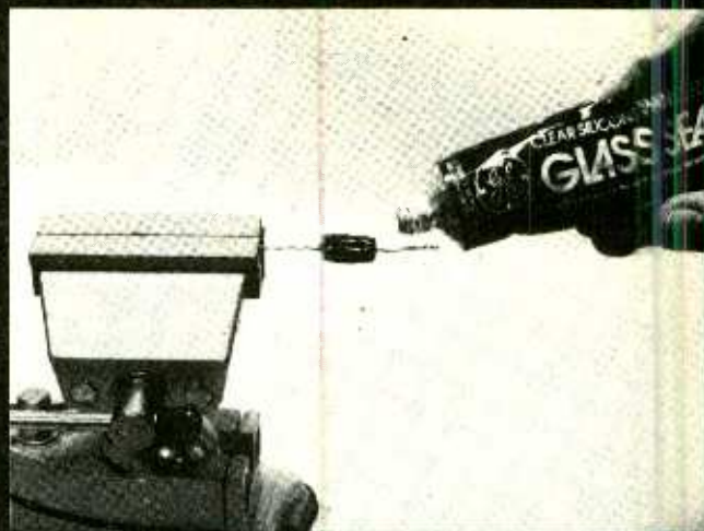
If you use a resistor as the form for a coil wound with very fine wire you must encapsulate the coil to prevent the turns of wiring from being displaced, or damaged in handling. A coat of RTV Silicon adhesive is even superior to “coil cement”.
