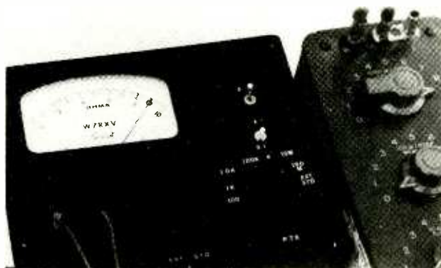
THE AUTHOR had access to a standard resistance box, providing him with practically unlimited selection of precision resistance values to adjust and test each resistance range at many points. You can do it with as few as one precision resistor.
