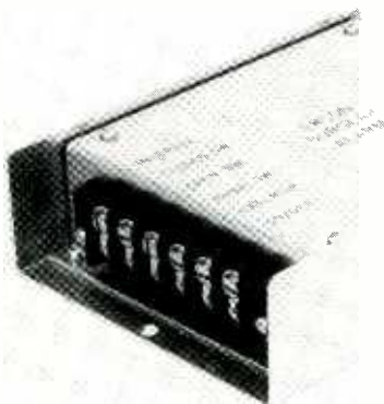
FIG. 3—EXTERIOR VIEW OF THE CONTROL BOX. The enclosure is 1.4 x 3.8 x 6 inches—easy to conceal from prying eyes.
