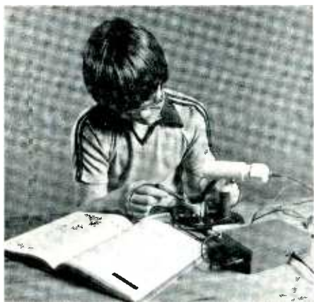
FIG. 5—PLASTIC PIPE forms a handy housing for probes and testers. (Photo; courtesy of American Technical Society)
