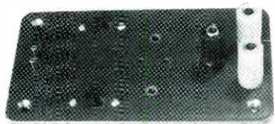
PLASTIC project box chassis lid with all of the top hardware in place.
