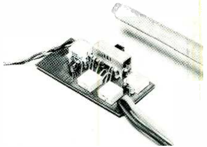
COMPONENT SIDE OF THE BOARD with all parts in place. Note that resistors are mounted upright.
