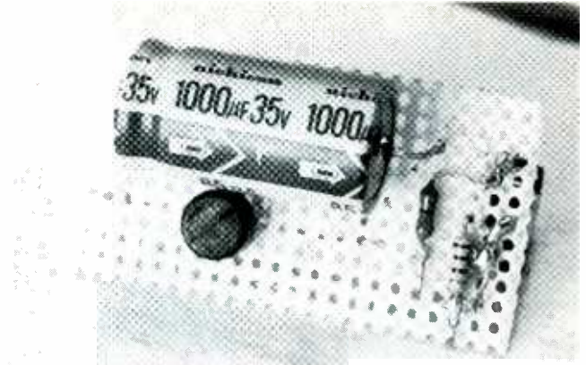
MOST OF THE CIRCUITRY fits on a small perforated board. The bridge rectifier is just below the capacitor.
