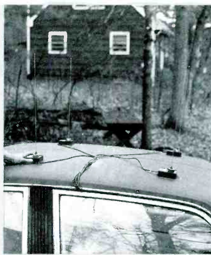
FIG. 6—DIRECTION FINDING using Doppler System's four matched quarter-wave whips, shown in (a), are supported on magnetically mounted bases for mobile operation. In (b), four collapsible antennas are mounted on a sturdy platform, on top of the author's roof.
