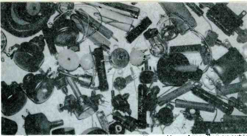
FIG. 1—THERE ARE MANY DIFFERENT resistor compositions and types. Among them are carbon, film, wirewound, cermet, and conductive plastic.
