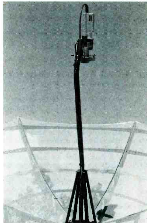
FEED-SUPPORT ARM places the feed and LNA (or LNB/LNC) at the focal point of the dish. The feed arm adjusts in and out to ensure precise setting for maximum signal.
