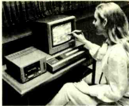
FIG. 5—COMPUTER-GENERATED GRAPHICS can be combined with single video frames on this terminal. An ordinary cassette tape is used to store the finished color images along with a sound track.
