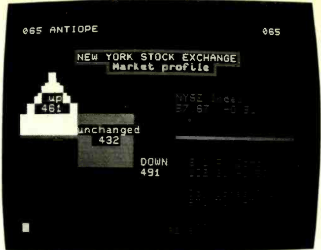
FIG. 3—ANTIQPE, THE FRENCH videotex system, uses a parallel-attribute system that permits higher-quality graphics.
