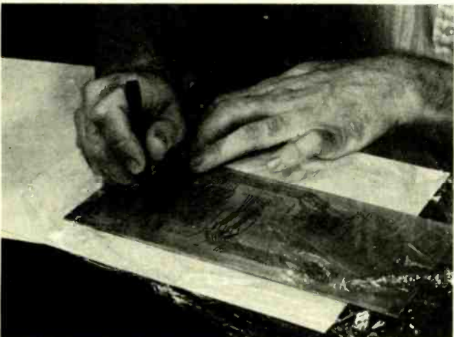
FIG. 6—PLASTIC KITCHEN WRAP is used to protect sections of the board that you are not working on from skin oils and smudging.
