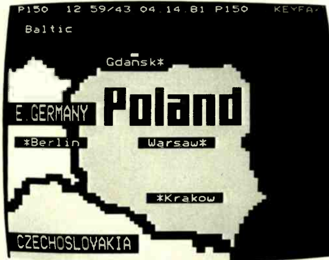
FIG. 2—THE BLACK LINES between different-colored areas are characteristic of the serial-attribute system used by Prestel.
