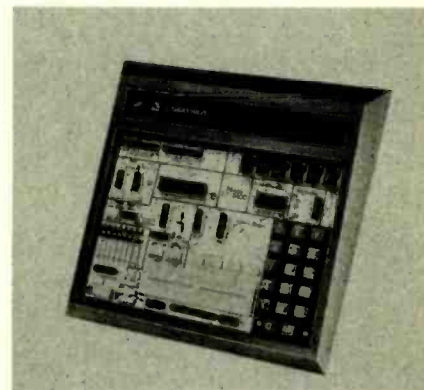
FIG. 5—A BUILT-IN solderless breadboard is among the features of the ET-3400 computer trainer from Heath.
