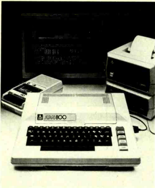
THE ATARI 800. Top opens to accept plug-in modules.
