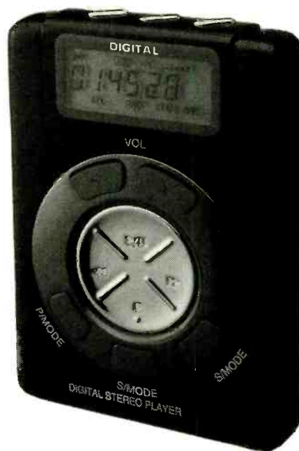
THE FIRST PORTABLE MP3 player still seems to be the best. Diamond's Rio PMP300 can hold 60 minutes of audio and will run for 12 hours on a single AA battery.
