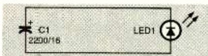
Fig. 1. Don't be fooled by the simplicity of the solar dosimeter's circuit—it is surprisingly accurate for such a low-cost device.
