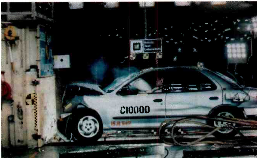
NOT ONLY WILL AIR BAGS DEPLOY in frontal crashes in many 1999 General Motors cars, but five seconds of critical pre-crash data will be recorded that could help reconstruct the accident and provide information for designing safer vehicles.
