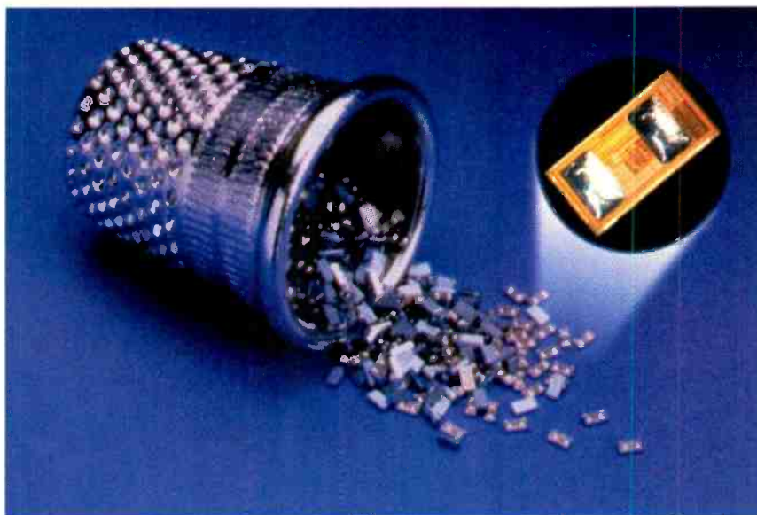
SHOWN HERE IS A THIMBLEFUL OF 1-Wire chips (actual-size), and in the upper right corner is a chip magnified many times.
