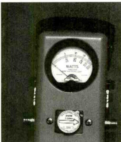
Fig. 9. The Bird Electronics Model 43 RF wattmeter is an old war horse that has served the author well over the years (photo courtesy of Bird Electronics Corporation).
