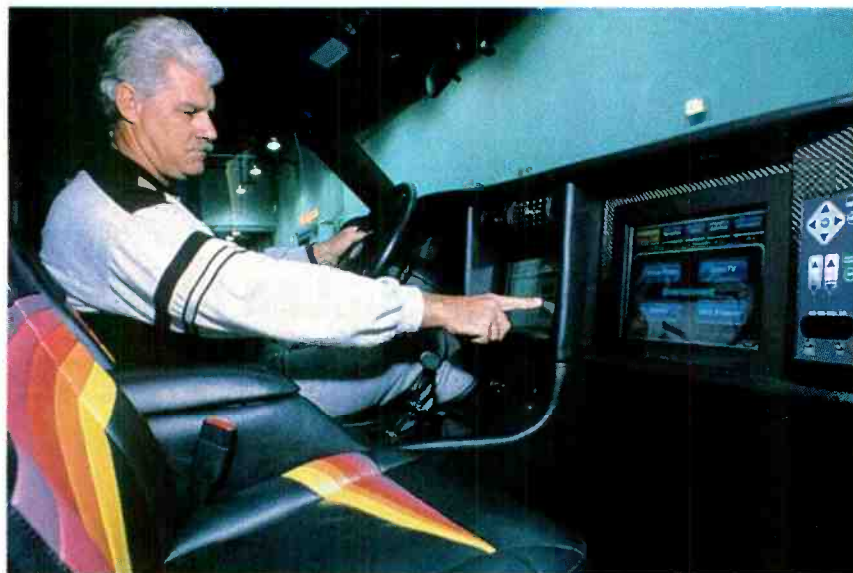
DRIVERS CAN ACCESS all the Network Vehicle's features using spoken commands or the reconfigurable touch-screen command console on the dashboard, located between the driver and passenger seats.
