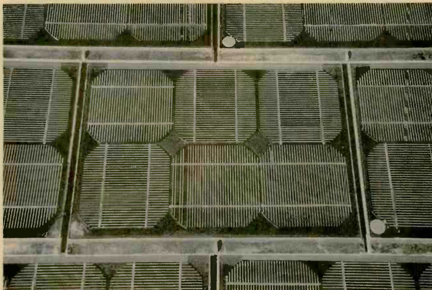
More appealing in appearance than conventional solar-power arrays, each individual SunSlate roofing tile, with a photovoltaic cell mounted on it, produces 12.5 watts. The tiles are nailed on to a structure just like conventional shingles
