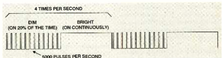
FIG. 4 —THE MODULATOR IN FIG. 3 VARIES the brightness of the bulb by changing the duty cycle of a squarewave. The pulse rate in the dim state is so fast that the filament does not flicker.
