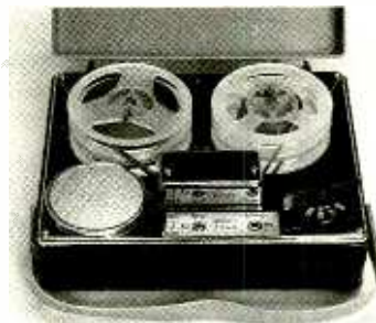
Fig. 10. Acme Model 1500 recorder. A modest 3-inch reel machine, using "rim drive" and a swing-out permanent magnet to erase previous recordings when in the record mode.
