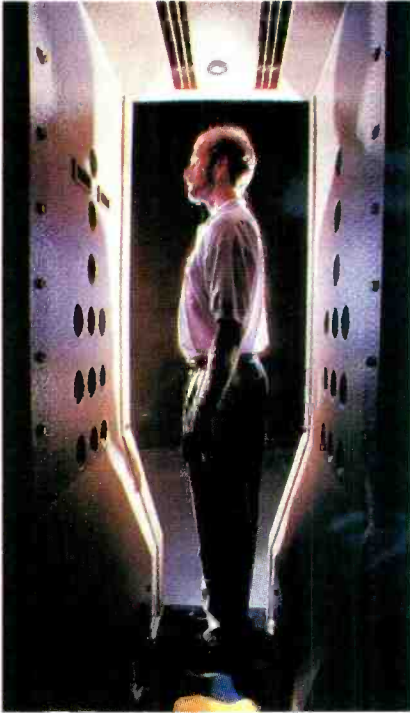
IN THE EXPLOSIVES-DETECTION PORTAL, a "puff" of air is blown over a person and an air sample is collected and analyzed by a spectrometer. (Sandia National Laboratories)
