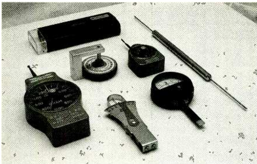
Fig. 5. Here are various measurement tools used to check tensions, speed, and wear.
