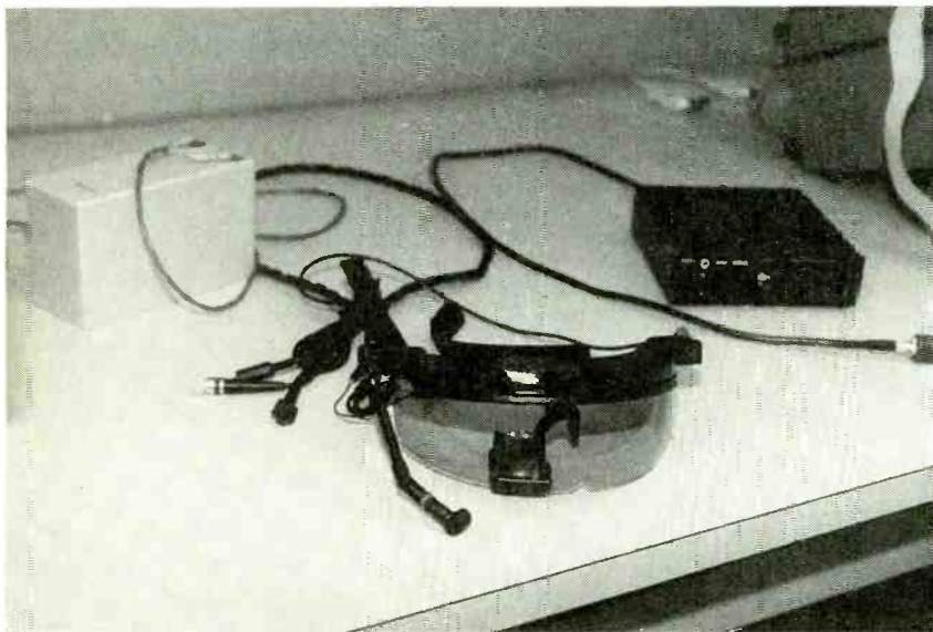
The Medic-Cam visor holds the tiny TV camera (upper right side of visor), TV monitor (center of visor in front of medic's eyes) and microphone. In the background are the control unit (right) and battery (left) plus associated cabling.
