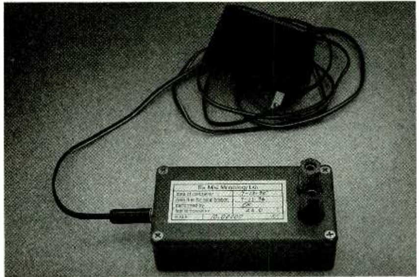
THE COMPLETED VOLTAGE STANDARD ready to serve as the first part of the Mini Metrology Lab.
