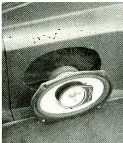
FIG. 11—IN A HATCHBACK CAR, rear speakers can be mounted on the panels in the hatch area.
