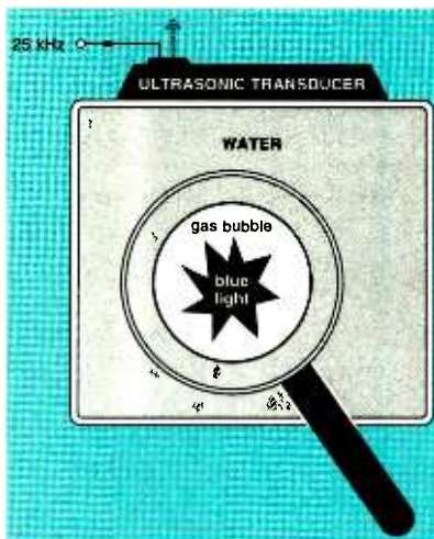
FIG. 1—SONOLUMINESCENCE results when ultrasonic waves become spherically focused to extremely high intensity. The center of a tiny air or gas bubble may get so hot that it emits ultra-short pulses of blue or ultraviolet light!
