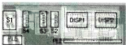
FIG. 6—PARTS PLACEMENT DIAGRAM for switch/display circuit board.
